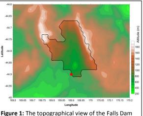
Catchment. The red point is the location of dam wall. The outlined area represents the area over which rainfall will flow into the Falls Dam lake.
